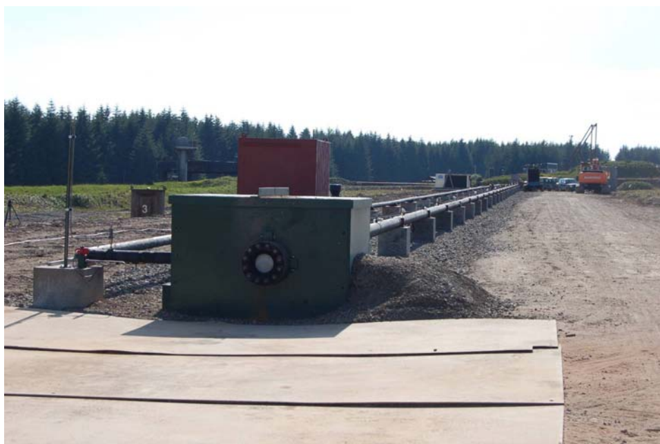
Figure 3 Photo of the shock tube test rig
