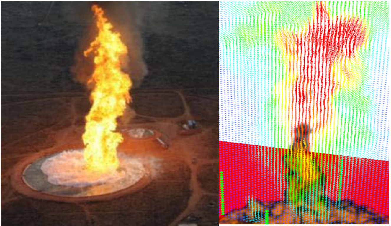
Figure 1 Photograph of Phoenix test 2 (Blanchat et al. , 2011) showing 83 m diameter pool and 56 m diameter fire (left), and sample results from an FDS simulation showing radial velocity sampling positions (right)
